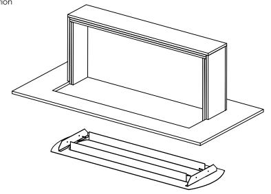
4. Prepare heater for installation Attach mounting brackets to both ends of heater with supplied fasteners
