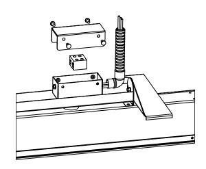
7. Raise one side of heater up into the ceiling box & then raise whole heater into cavity.
