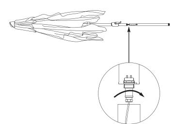
Insert bottom pole into canopy/mainframe pole. Line up button with hole and snap into place.
