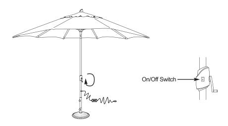
To tilt, continue to turn the crank to desired position.
