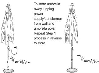
**Note:** During disassembly, it is important to loosen knob of plug *inside* umbrella poles **first**, then remove bottom pole from mainframe/canopy. If not, the wire will be split and result in damage to lighting.
