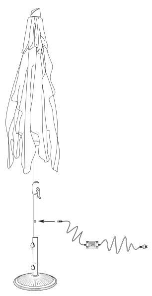
**Note:** The transformer output power is 12V. It is normal for transformer to get warm after long period of use. Avoid sun on power supply/transformer to increase lifetime use.
